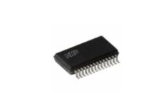
UBA2035TS/N1,118 NXP USA Inc. IC DVR HF FULL BRIDGE 28-**SSOP**
