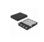
STL120N2VH5 STMicroelectronics MOSFET N-CH 20V 120A POWERFLAT56
