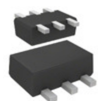
DMG504010R Panasonic Electronic Components TRANS NPN/PNP 50V 0.1A SMINI6
