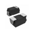
**GS1ME-TP** Micro Commercial Co DIODE GEN PURP 1KV 1A DO214AC
