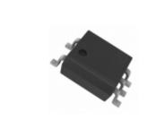
PC400J00000F Sharp Microelectronics OPTOISO 3.75KV OPEN COLL 5MFP
