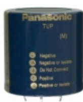
ECE-P2WP821HA Panasonic Electronic Components CAP ALUM 820UF 20% 450V SNAP
