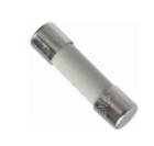
5HT 1-R Bel Fuse Inc. FUSE CERAMIC 1A 250VAC 5X20MM
