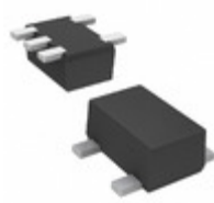
DMC561070R Panasonic Electronic Components TRANS 2NPN PREBIAS 0.15W SMINI5
