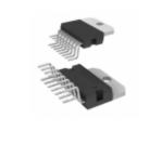
TDA7295 STMicroelectronics IC AMP AUDIO 80W AB MULTIWATT15
