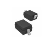
SMV1232-011LF Skyworks Solutions Inc. SOD 323 N-TYPE SINGLE LEAD
