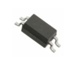
PC3H5J00000F Sharp Microelectronics OPTOISO 2.5KV DARLNG 4-MINI-FLAT
