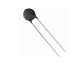
**SL12 25003** Ametherm ICL 25 OHM 15% 3A 12MM
