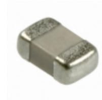
W2F43A1018AT1F AVX Corporation CAP FEEDTHRU 100PF 25V NP0 0805
