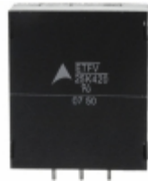
ETFV25K420E4 EPCOS (TDK) VARISTOR 680V 20KA RADIAL
