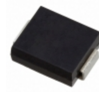
MXLSMCJ9.0CA Microsemi Corporation TVS DIODE 9VWM 15.4VC DO214AB
