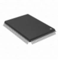
MB90F342APF-GE1 Cypress Semiconductor IC MCU 16BIT 256KB FLASH 100QFP
