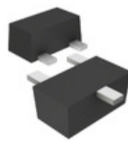
DRA9143E0L Panasonic Electronic Components TRANS PREBIAS PNP 125MW SSMINI3
