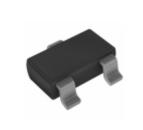
FMMTL720TC Diodes Incorporated TRANS PNP 40V 1A SOT23-3
