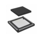
SI2113-A10-GM Silicon Labs IC SAT TV RCVR DVB-C 48-QFN
