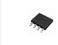
BD9161FVM-TR Rohm Semiconductor IC REG BUCK ADJ 0.6A SYNC 8MSOP
