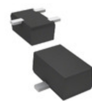
DRA5124E0L Panasonic Electronic Components TRANS PREBIAS PNP 150MW SMINI3
