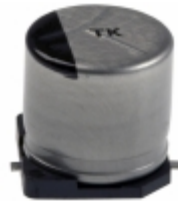
EEE-TK2A331AM Panasonic Electronic Components CAP ALUM 330UF 20% 100V SMD
