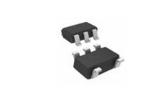
LK112M33TR STMicroelectronics IC REG LDO 3.3V 0.15A SOT23-5
