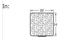
4049PA51H00400 Laird Technologies GASKET FAB/FOAM 6.35X101.6MM SQ
