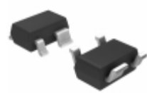
BF904WR,115 NXP USA Inc. MOSFET N-CH 7V 30MA SOT343
