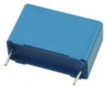
B32523Q335K EPCOS (TDK) CAP FILM 3.3UF 10% 63VDC RADIAL
