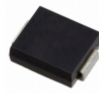
MXLSMCJLCE14AE3 Microsemi Corporation TVS DIODE 14VWM 23.2VC DO214AB
