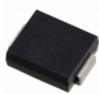
MXLSMCJLCE12A Microsemi Corporation TVS DIODE 12VWM 19.9VC DO214AB
