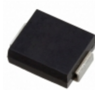
MXLSMCJLCE12AE3 Microsemi Corporation TVS DIODE 12VWM 19.9VC DO214AB
