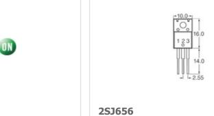
**ON Semiconductor** MOSFET P-CH 100V 18A TO-220ML
