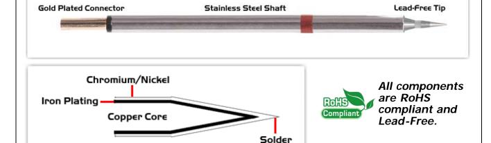
Easy Braid Co. tip cartridges will typically idle within a temperature range of +/-1.1°C. However, there is variation in idle temperature across tip geometries within an individual temperature series. Easy Braid Co. offers a wide variety of tip geometries from 0.25mm fine point tip to 5mm chisel. The length and geometry of a tip will have an influence on the tip idle temperature. To accurately measure idle temperature it will depend greatly on the measurement method,
