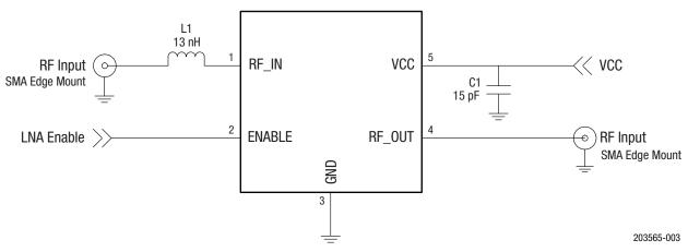
Figure 3. SKY65623-682LF Application Schematic
