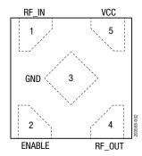
Figure 2. SKY65623-682LF Pinout (Top View)
