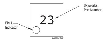
Figure 8. SKY65623-682LF Typical Part Marking (Top View)
