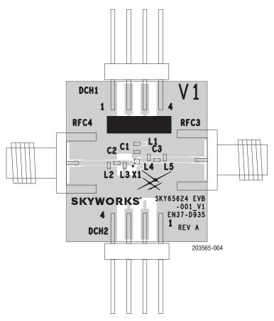
Figure 4. SKY65623-682LF Evaluation Board Assembly Diagram
