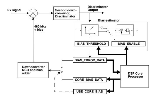
Figure 5. AFC Loop and Processor Control
