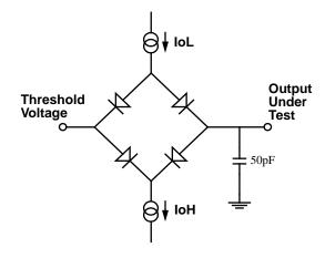
Figure 5. Test Load Diagram
