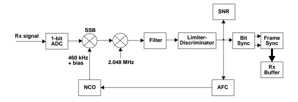
Figure 2. Demodulator Block Diagram
