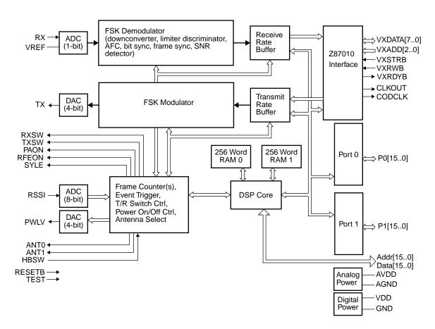
Figure 2. Z87001 Functional Block Diagram
