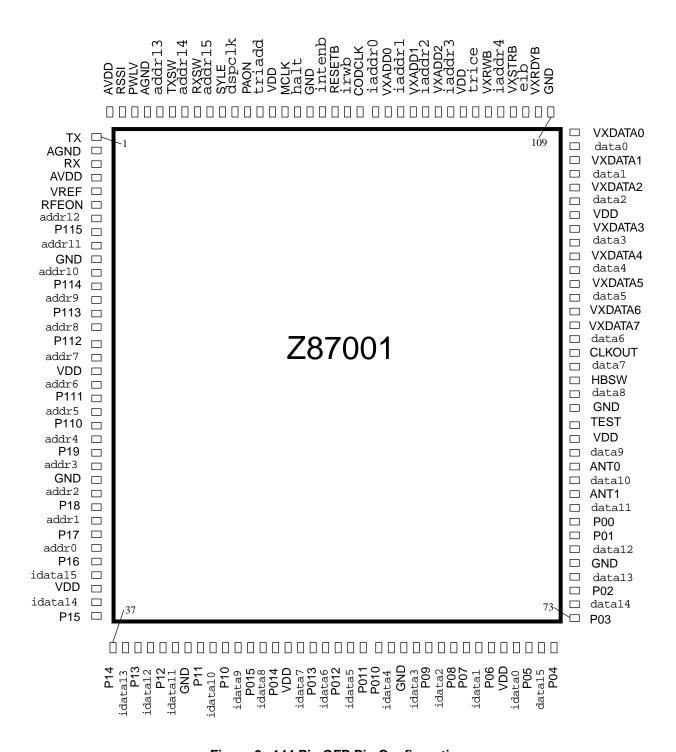
Figure 3. 144 Pin QFP Pin Configuration
