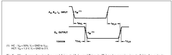
Fig.6 Waveforms showing the word A inputs  $(A_n)$ , word B inputs  $(B_n)$  and expansion inputs  $(I_n)$  to the outputs  $(Q_n)$  propagation delays and the output transition times.
