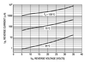
**Figure 2. Typical Reverse Current**
