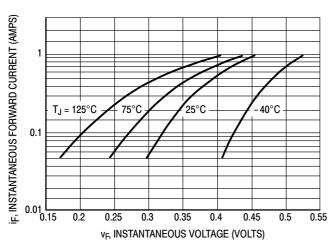
Figure 1. Typical Forward Voltage
