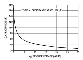
Figure 3. Typical Capacitance
