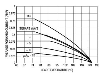
Figure 4. Current Derating (Lead)
