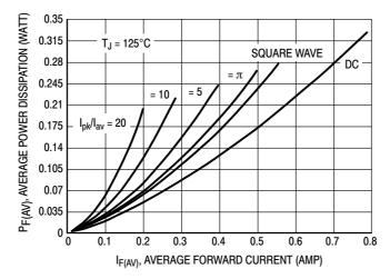
Figure 5. Power Dissipation
