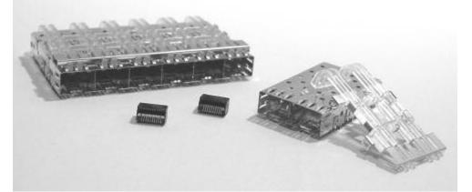
The Ganged SFP product line allows for single row, high density port designs to maximize the horizontal I/O space. The design allows for belly-to-belly orientation to maximize port density. The lateral port-to-port spacing is minimized to 14.25mm, compared to 16.25mm required spacing between single port cages. Port configurations include 1x2, 1x4 and 1x6, with lightpipes optional.
