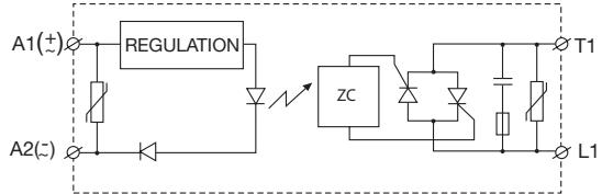
Note: Varistor on output is not included in the RGS1A69... models
