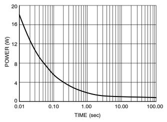
Figure 10. Single Pulse Power
