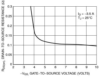
Figure 3. On-Resistance vs. Gate-to-Source Voltage
