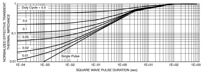
Figure 9. Normalized Thermal Transient Impedance, Junction-to-Ambient
