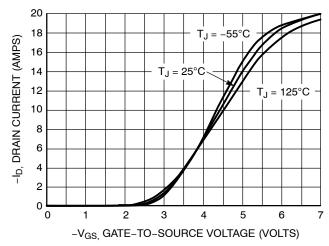
Figure 2. Transfer Characteristics
