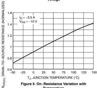
Figure 5. On-Resistance Variation with **Temperature**
