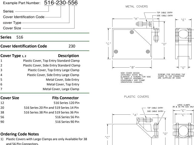
Metal Covers with side entry may be converted to top 2) entry by removing side plate and changing clamp orientation.
