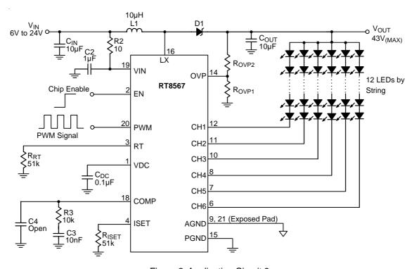
Figure 2. Application Circuit 2
