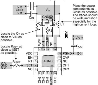
Figure 3. PCB Layout Guide
