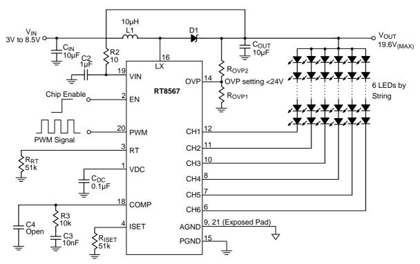
Figure 1. Application Circuit 1
