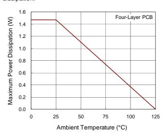
Figure 2. Derating Curve for RT8567 Package
