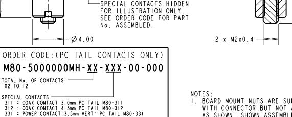
I. BOARD MOUNT NUTS ARE SUPPLIED WITH CONNECTOR BUT NOT ASSEMBLED AS SHOWN. SHOWN ASSEMBLED FOR ILLUSTRATION ONLY.
