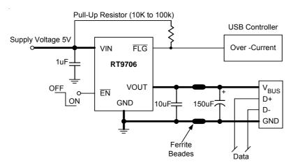
**Note:** A low-ESR 150 $\mu$ F aluminum electrolytic or tantalum between VOUT and GND is strongly recommended to meet the 330mV maximum droop requirement in the hub V<sub>BUS</sub>. (see Application Information Section for further details)
