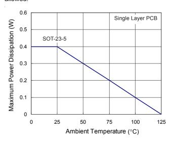
Figure 2. Derating Curves for RT9706 Package
